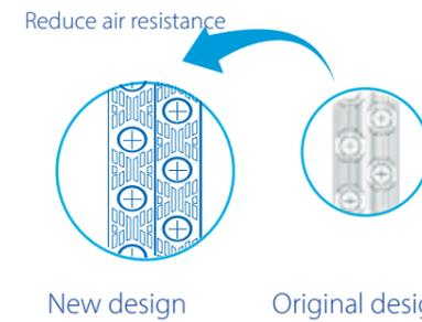
Hydrophilic film fins and inner-threaded copper pipes optimize heat exchange efficiency.
