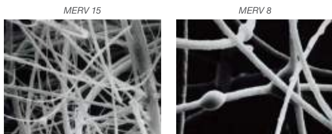
MERV 15 vs. MERV 8 media under 2000x magnification
