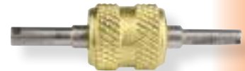
92820 Valve Core Tool Double ended for removing and installing both standard and large bore valve cores
