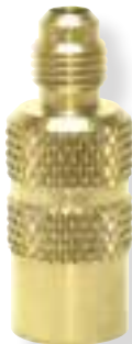
92863 R-410A Mini-Split Adapter 5/16"(1/2"-20) Female with Adjustable Depressor x 1/4" Male with Valve Core
