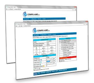
Compu-Aire Inc. advanced microprocessing control system provides access to our equipment through building management system (BMS) supporting industrial standard protocols including Modbus, BACnet, and LonWorks. This ensures easy access to the remote management of the unit via modem and internet.
