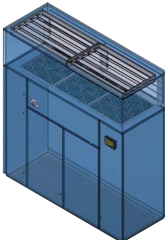
(iii) Downflow With Top Return With Outside Air Economizer
