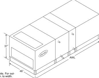
NOTES:1. Dimensions are shown for indoor units. For outdoor units add 4 in. to height and 3 in. to width.2. Height dimensions include 6-in. base rail.
