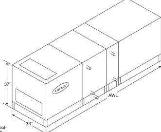
NOTES:1. Dimensions are shown for indoor units. For outdoor units add 4 in. to height and 3 in. to width.2. Height dimensions include 6-in. base rail.
