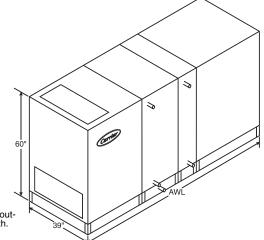
NOTES:1. Dimensions are shown for indoor units. For out-door units add 4 in. to height and 3 in. to width.2. Height dimensions include 6-in. base rail.
