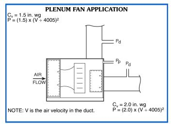
The 39M Series airfoil and forward-curved fans are tested as part of a system with straight discharge ductwork, and the fan ratings are based on this duct design. When designing ductwork in the field, it is important to use a straight discharge duct of the correct dimensions to obtain maximum fan performance. Straight ductwork helps the airflow to develop a uniform velocity profile as it exits the fan and allows the velocity pressure to recover into static pressure. See the figure below.
