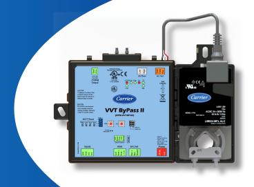
The VVT Bypass II controller is used to regulate the supply duct static pressure for a variety of pressure-dependent VVT applications and allows constant volume HVAC equipment to provide zone level temperature control. This advanced controller features a separable, brushless actuator and an integral pressure sensor for reliability and longevity. It also features native BACnet communications and plug-and-play connectivity to the Carrier i-Vu Building Automation System.
