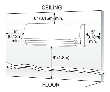
Fig. 3 — Indoor Unit Clearances
