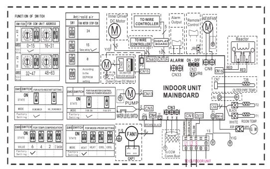
Fig. 7 - Wiring Diagram Sizes 09 - 12
