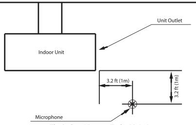
Fig. 6 – Sound Pressure Testing Method
