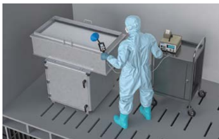
Bench testing of a HEPA/ULPA filter
